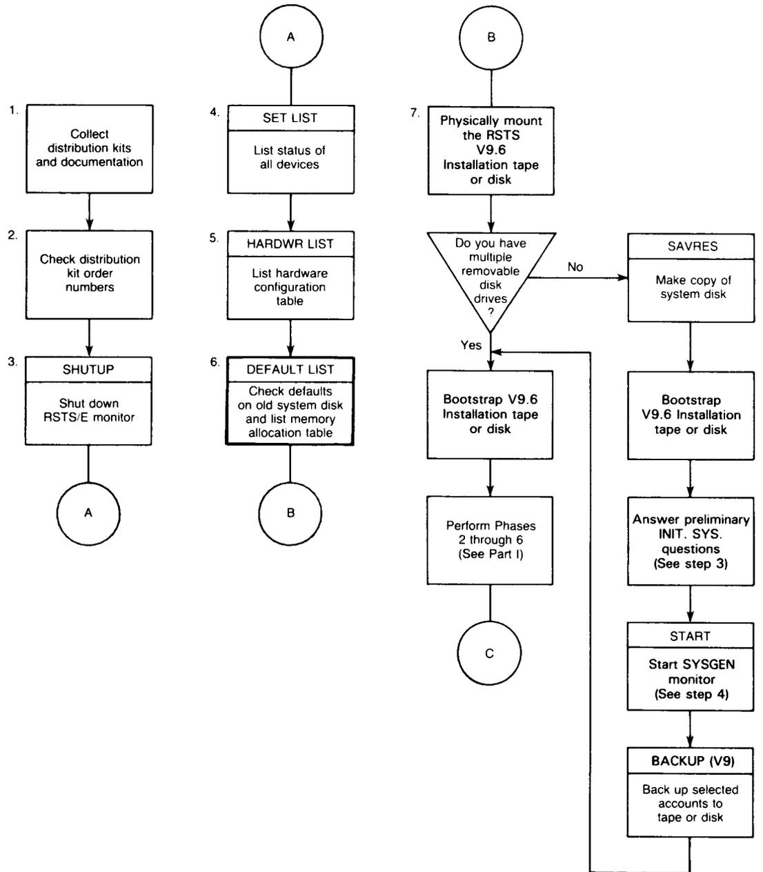
**Figure 3: System Upgrade Flowchart**
