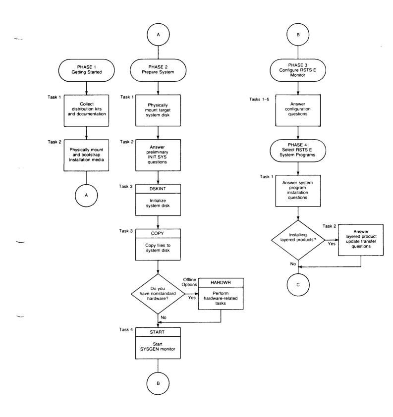
Figure 1: System Installation Flowchart
